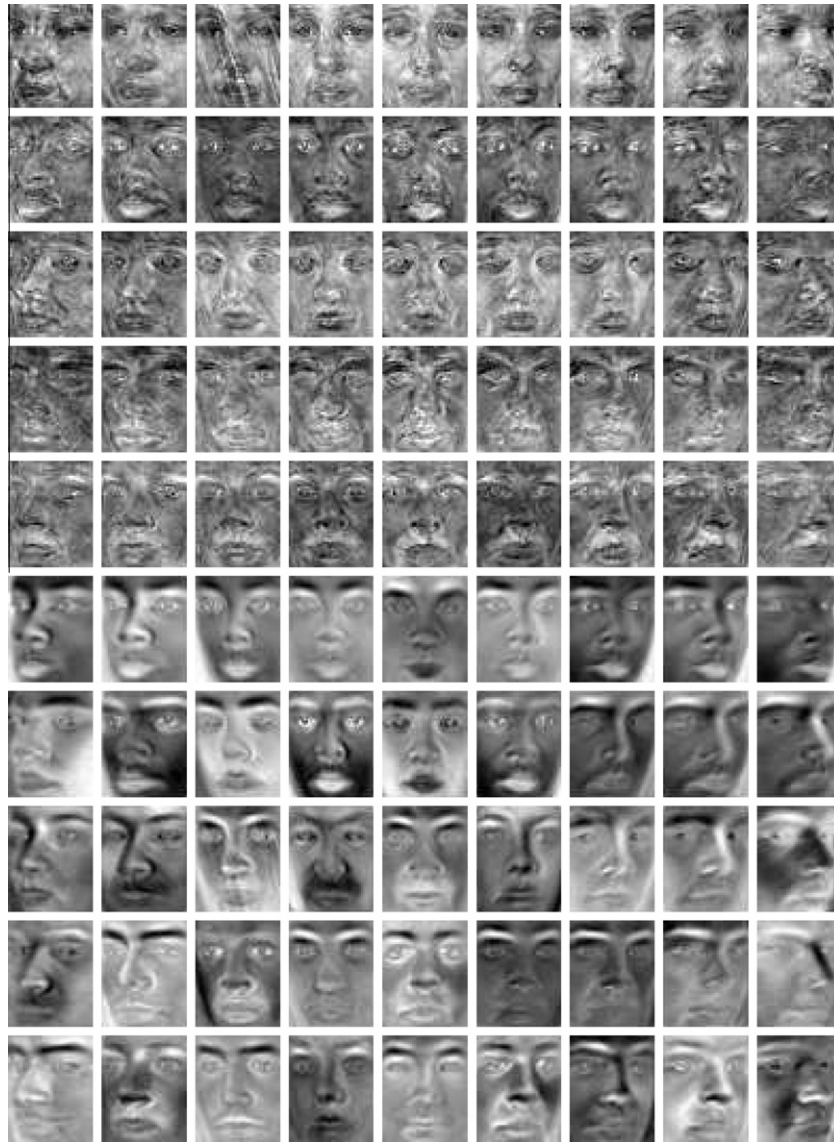
Fig. 10. Projector bases corresponding to top eigen-values obtained using CCA (first five rows) and PCA [32] (bottom five rows) obtained using 100 subjects from FERET. CCA projectors are learned using all the poses simultaneously and PCA projectors are learned separately for each pose. Each row shows the projector bases of the pose for equally indexed eigen-value. Observe that, projector bases are hallucinated face images in different poses and the CCA projector bases look like rotated versions of the same hallucinated face but there is considerable difference between PCA projectors. This picture visually explains the presence of correlation in the latent CLS space using CCA and its absence using PCA.
